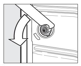
■ Use the combination wrench supplied to turn the left-hand shipping rod 90°, and then
